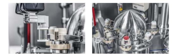
The ready-to-fill AT-Closed Vial<sup>®</sup>, organized in AT-Nest<sup>™</sup>, and other consumable materials are introduced into the main chamber via a rapid decontamination airlock, while the bulk product is aseptically connected to the main chamber of the isolator thanks to the use of the AT-Port<sup>™</sup> system, integrated on the isolator wall. Such configuration allows the bulk product to be homogenized and cooled.
