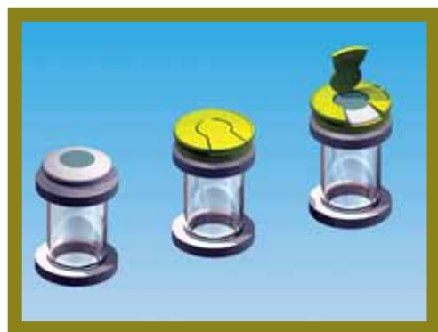
Figure 3: The sterile, ready-to-fill vial is delivered uncapped (left). After filling, the vial is capped (middle) inside an isolator. To use the vial, the central part of the flip-top cap is removed (right), exposing the large puncture area that has been kept sterile by the circular rib.
