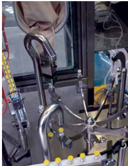
Figure 6: Overview of the filling area in a clinical line. Inside the RABS, a wheel moves the vials to each filling step: the filling with the needle piercing the stopper (top right); the resealing of the stopper with a laser (top left); and capping (bottom left) before the vials exit the RABS.
