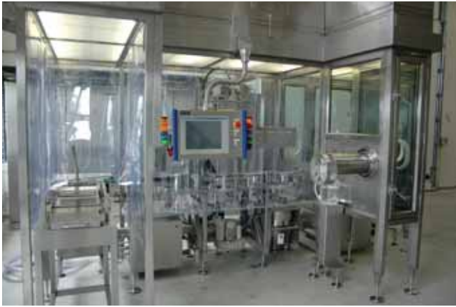
Figure 5: Overview of a clinical machine with the loading and electronic beam steps conducted under a soft-wall laminar airflow (on the left) and the filling steps (filling, laser resealing, and capping) conducted in a restricted access barrier system (RABS, on the right).
