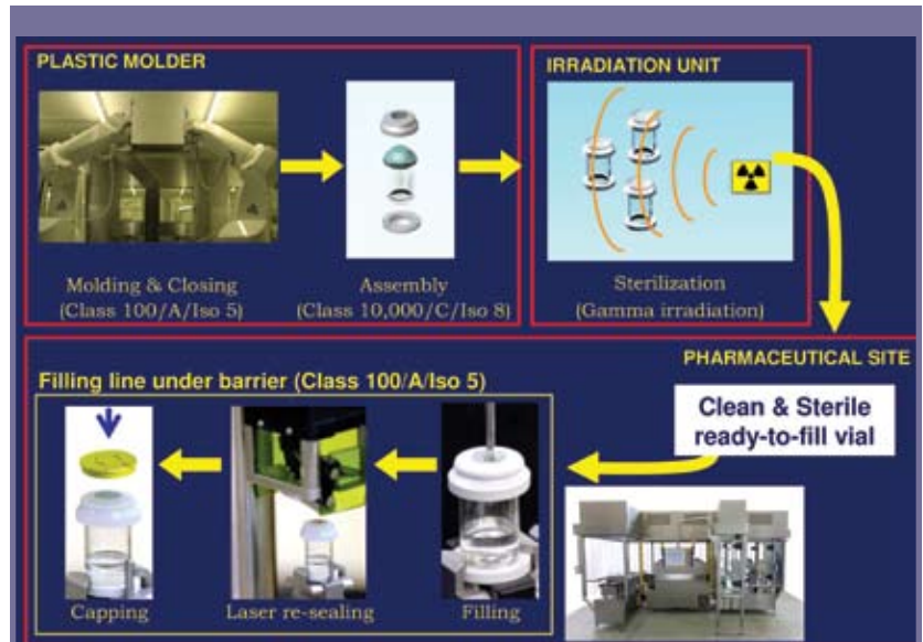
Figure 1: Closed vial process: Vial bodies and stopper are molded in ISO 5 (Class 100/Grade A) environment and immediately assembled by robot before the top and bottom rings are added; after packaging, the vials are gamma-irradiated; at the pharmaceutical site, vials are filled with a needle passing through the stopper, which is then laser resealed; and finally, capping is completed.
